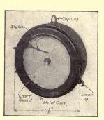
Fig. 28.—A graphic demand meter (General Electric, Type G-2).
